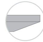
Chamfered edge with 3mm radius
